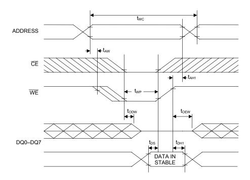
Figure 6. MEMORY WRITE CYCLE TIMING, CHIP-ENABLE CONTROLLED (Notes 5, 7, 8, 10, 11, 12, and 13)
