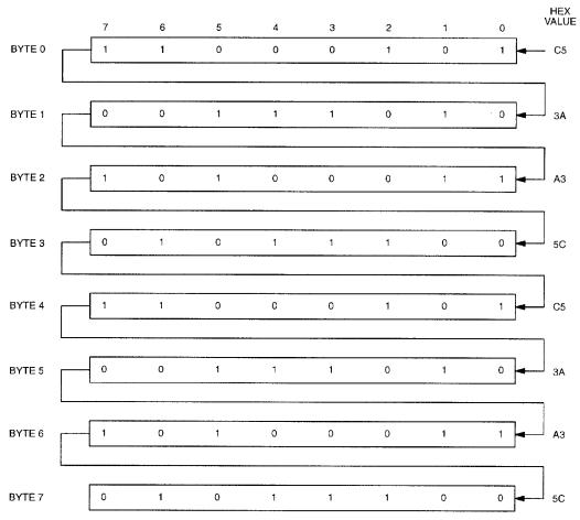
**Note:** The pattern recognition in hex is C5, 3A, A3, 5C, C5, 3A, A3, 5C. The odds of this pattern being accidentally duplicated and causing inadvertent entry to the phantom clock is less than 1 in 10<sup>19</sup>. This pattern is sent to the phantom clock LSB to MSB.
