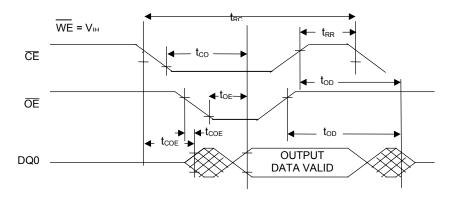
Figure 8. WRITE CYCLE TO PHANTOM CLOCK
