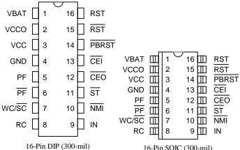
16-Pin DIP (300-mil) See Mech. Drawings Section 16-Pin SOIC (300-mil) See Mech. Drawings Section
