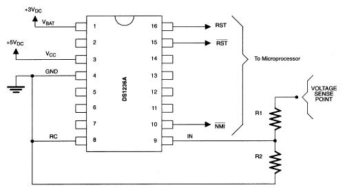
EXAMPLE 1: 5-VOLT SUPPLY, R2 = 10k OHM,  $V_{\text{SENSE}} = 4.80$  VOLTS  $\therefore 4.80 = \frac{\text{R1} + 10\text{k}}{10\text{k}} \text{ X 2.54} \qquad \text{R1} = 8.9\text{k OHM}$
