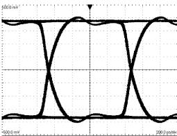
Figure 7. A 1.06 Gbps NRZ PRBS-7 After 2" Differential FR-4 Stripline V:100 mV / DIV, H:200 ps / DIV
