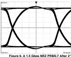
Figure 6. A 1.5 Gbps NRZ PRBS-7 After 2" Differential FR-4 Stripline V:100 mV / DIV, H:100 ps / DIV
