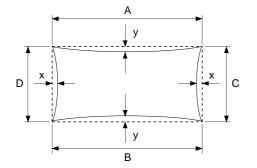
Right/left distortion = (4x)/(A + B)Up/down distortion = (4y)/(C + D)
