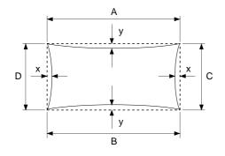
Right/left distortion = (4x)/(A + B)Up/down distortion = (4y)/(C + D)
