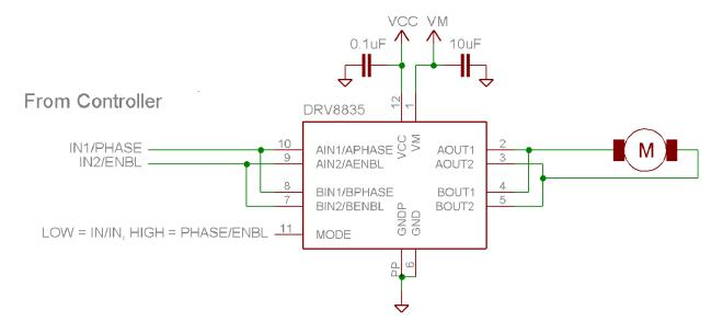
Figure 1. Parallel Mode Connections
