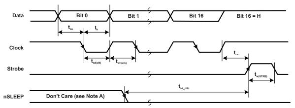
A. For initial setup, nSleep state can be "Don't care" before the tss\_min timing prior to the strobe.
