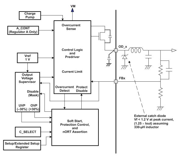
Figure 8. DC-DC Converter
