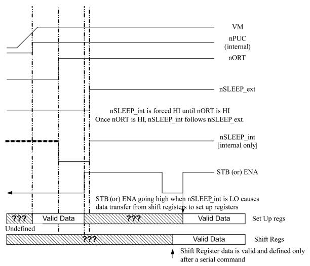
A. During startup (VM rising), internally nSLEEP de-asserted to HI, suppressing false data latching caused by a rising edge on the STB signal. nSLEEP will remain HI until nORT is released (120 ms after dc-dc regulators come up).
