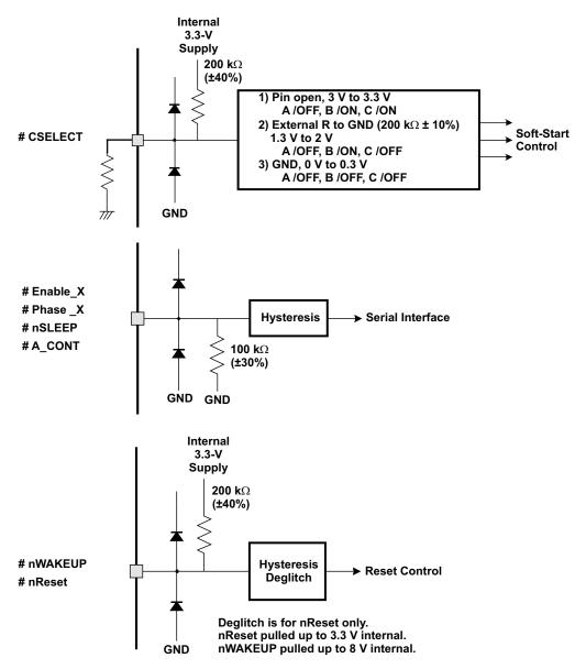
Figure 1. Input Pin Configuration
