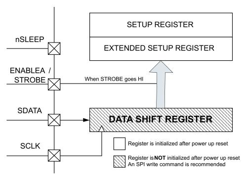
A. It is recommended that after initial power up sequence, a serial command be performed to clear undefined data in the internal shift register. This will help avoid latching undefined data into SETUP and EXTENDED SETUP registers. SETUP and EXTENDED SETUP registers are properly initialized during power up, but internal shift register is not initialized.
