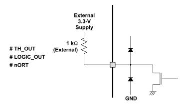
Figure 2. Open-Drain Output Pin Configuration
