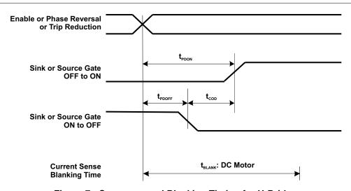
Figure 7. Crossover and Blanking Timing for H-Bridge
