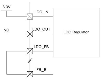
Figure 9. Unused LDO Recommended Connections
