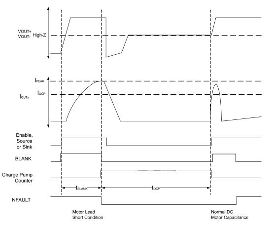
Figure 2. Overcurrent Control Timing
