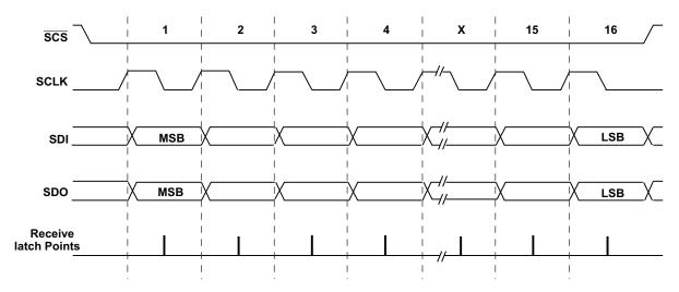
Figure 3. SPI Slave Mode Timing Diagram
