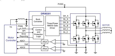
Figure 1. DRV8301 Simplified Application Schematic
