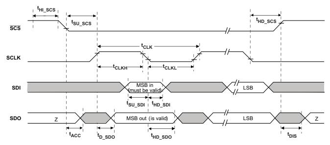
Figure 2. SPI Slave Mode Timing Definition
