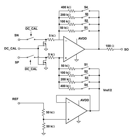
Figure 4. Current Shunt Amplifier Simplified Block Diagram
