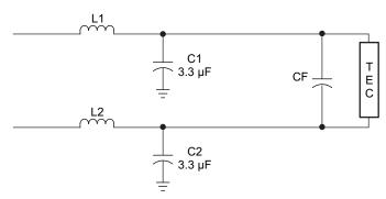
Figure 12. Second Order Butterworth Low-Pass Filter Configuration
