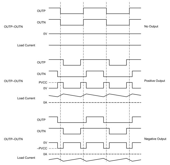
Figure 16. BD Mode Modulation
