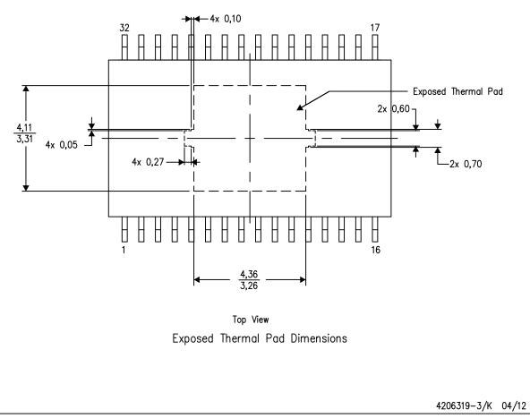
NOTE: All linear dimensions are in millimeters
