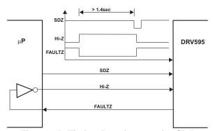
Figure 15. Timing Requirement for SDZ
