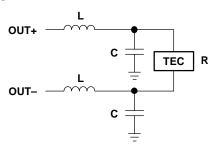
Figure 13. LC Output Filter
