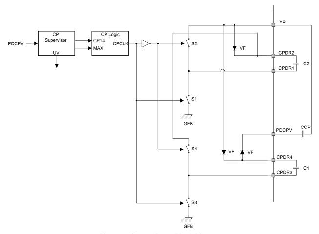
Figure 8. Charge Pump Block Diagram
