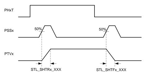
Figure 20. Settling Time Timing Chart (Sample and Hold Mode)
