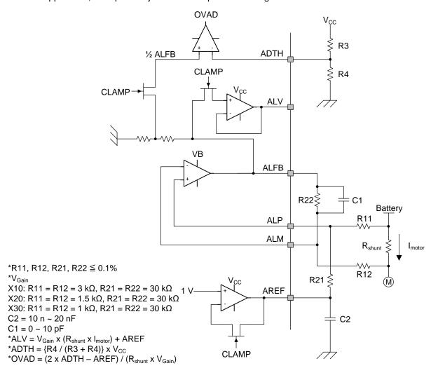
Figure 12. Motor Current Sense Block Diagram
