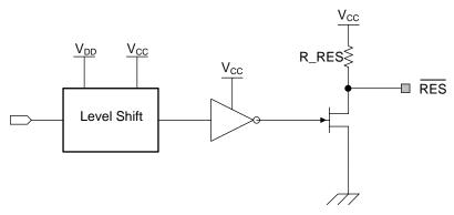
Figure 30. Output Buffer 3 Block Diagram
