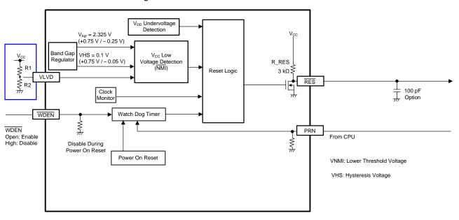
Figure 2. Watchdog Block Diagram
