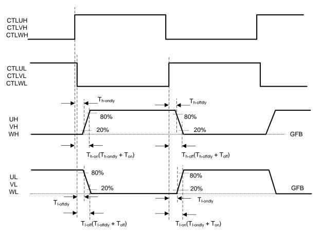
Figure 10. Delay Time from Input to Output
