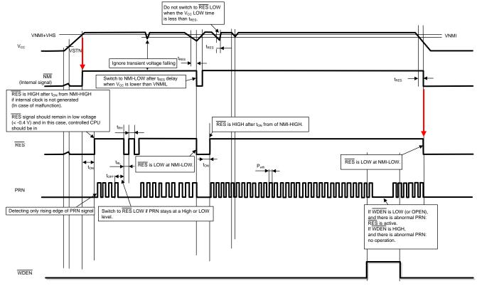
NOTE:  $\overline{\text{WDEN}} = \text{High}$ ,  $V_{CC}$  undervoltage condition sets  $\overline{\text{RES}} = \text{Low}$
