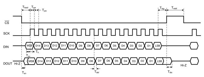
Figure 6. SPI AC Timing Definition
