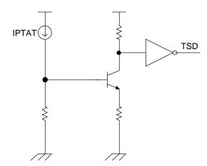
Figure 25. Thermal Shutdown Block Diagram
