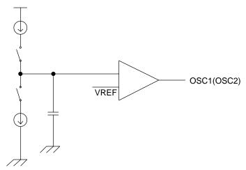
Figure 26. Oscillator Block Diagram
