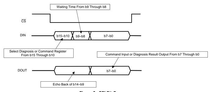
Figure 5. SPI Bit Sequence
