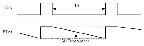
Figure 19. Holding Timing Chart
