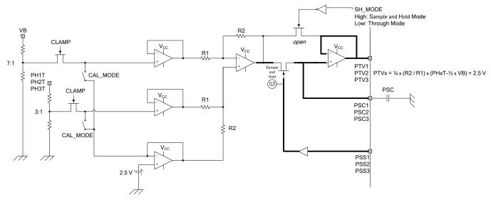
Figure 15. Sample and Hold Mode Block Diagram
