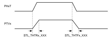
Figure 21. Settling Time Timing Chart (Through Mode)
