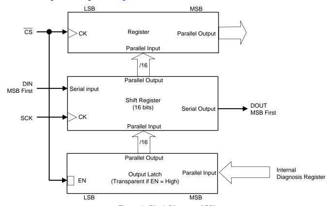
Figure 4. Block Diagram of SPI
