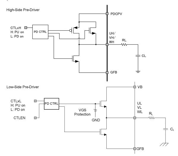
Figure 9. Pre-driver Block Diagram
