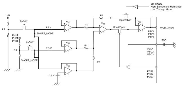
Figure 17. Short Mode (Optional) Block Diagram
