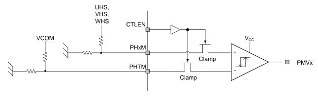
Figure 11. Phase Comparator Block Diagram
