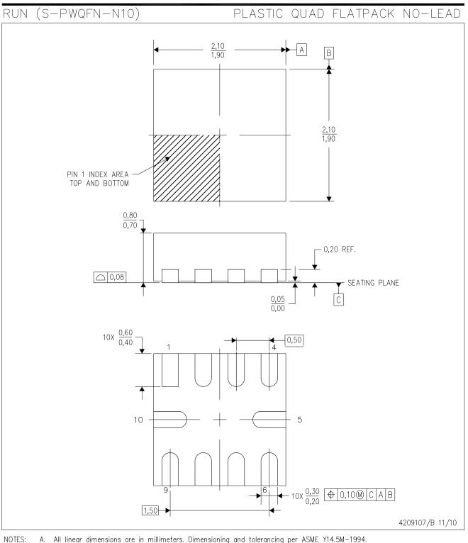
A. All linear dimensions are in millimeters. Dimensioning and tolerancing per ASME Y14.5M-1994.
