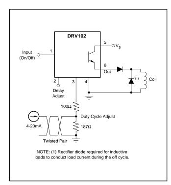
FIGURE 16. 4-20mA Input to PWM Output.
