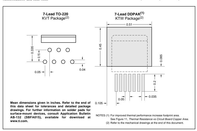
FIGURE 10. TO-220 and DDPAK Solder Footprints.
