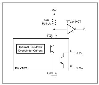
FIGURE 7. Non-Latching Fault Monitoring Circuit.
