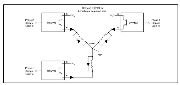
FIGURE 22. Three-Phase Stepper Motor Driver Provides High-Stepping Torque.
