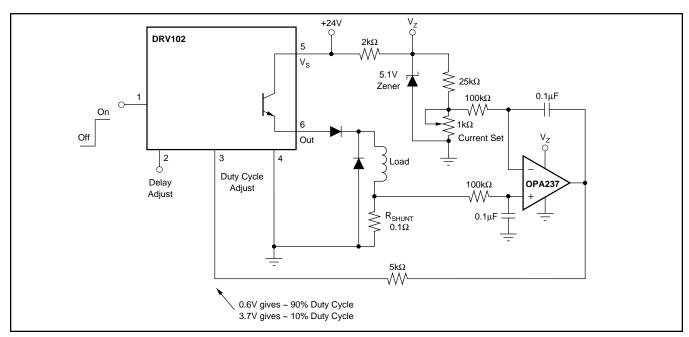
FIGURE 21. Constant Current Output Drive.
