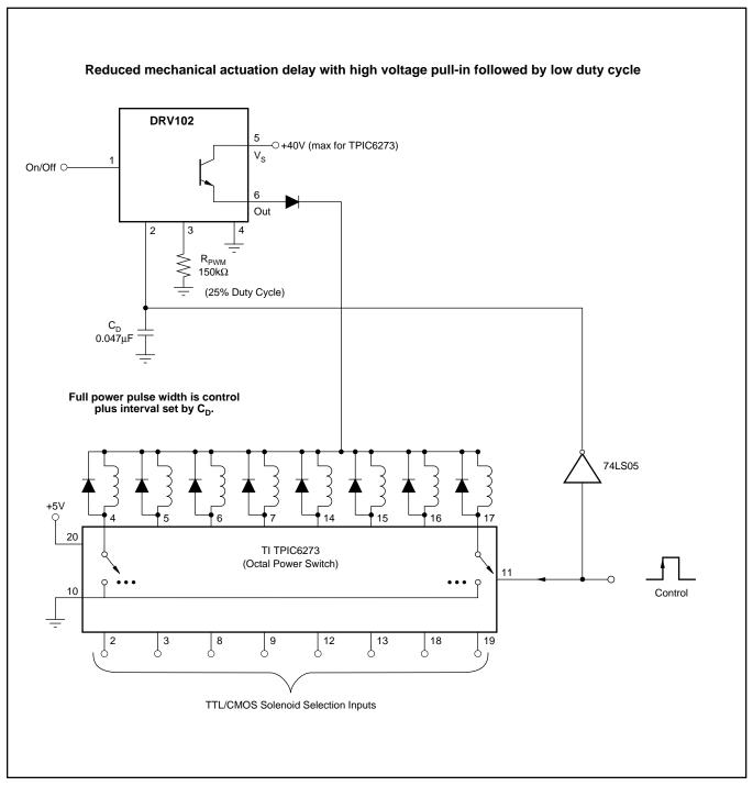
FIGURE 17. Improved Switching Time When Driving Multiple Loads.
