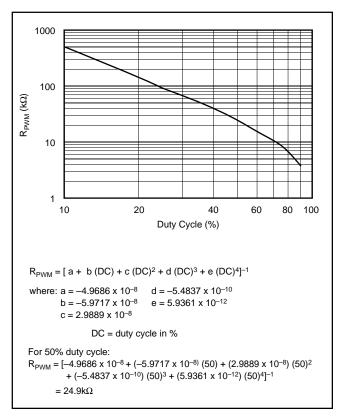
FIGURE 4. R<sub>PWM</sub> versus Duty Cycle.
