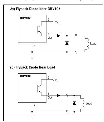
FIGURE 2. Location of External Flyback Diode.
