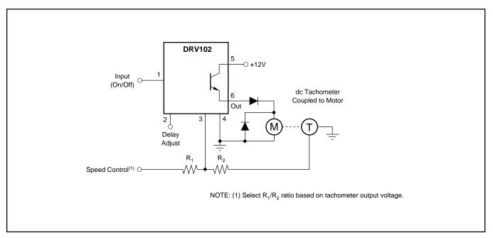
FIGURE 19. Constant Speed Motor Control.
