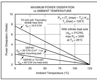
FIGURE 13. Maximum Power Dissipation versus Ambient Temperature.
