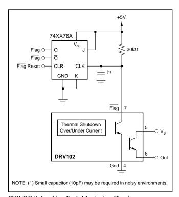
FIGURE 8. Latching Fault Monitoring Circuit.
