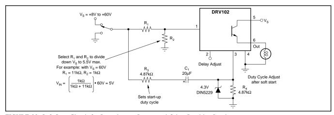
FIGURE 23. Soft-Start Circuit for Incandescent Lamps and Other Sensitive Loads.
