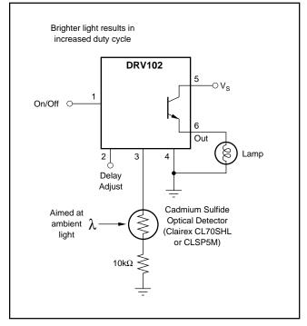
FIGURE 15. Instrument Light Dimmer Circuit.
