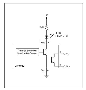
FIGURE 9. LED to Indicate Fault Condition.
