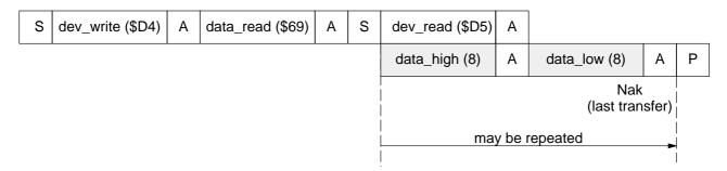
Fig. 7-5: Reading 16-bit data word(s) from the data register
