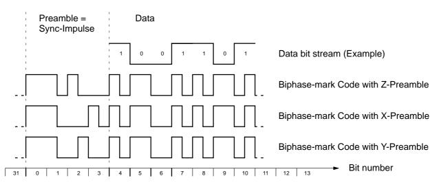
Fig. 6–5: Preamble and biphase-mark code specification (polarity may be changed)
