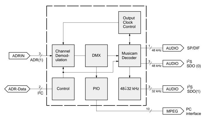
Fig. 1-2: DRP 3510A simplified block diagram
