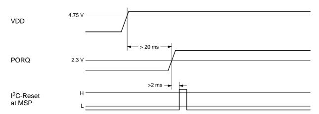
Fig. 12-8: Recommended power up sequence (24 MHz single crystal mode)
