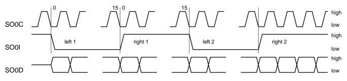
Fig. 6–3: Schematic timing of the SDO1 output interface
