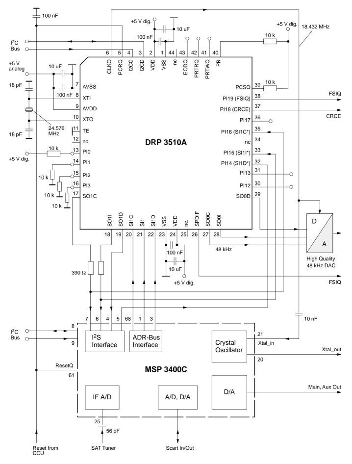
11.6. Typical ADR Application Circuit (DRP Application with 24 MHz Single Crystal Mode)
