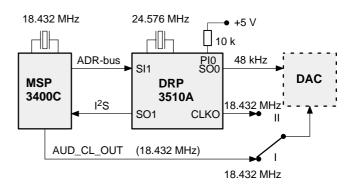
**Fig. 5–2:** Two crystal mode with 18.432 and 24.576 MHz crystal
