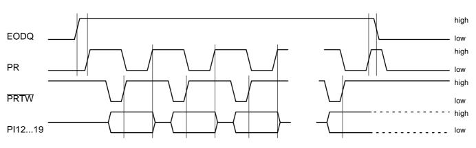
Fig. 6-4: Handshake protocol for getting MPEG data via PIO-DMA
