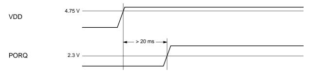
Fig. 12-6: Recommended power up sequence (dual crystal modes)
