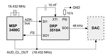
Fig. 5–4: Single crystal mode with 18.432 MHz
