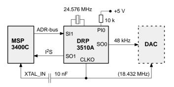
Fig. 5-3: Single-crystal mode with 24.576 MHz
