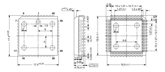
**Fig. 3–1:** 44-Pin Plastic Leaded Chip Carrier Package **(PLCC44)** Weight approximately 2.5 g Dimensions in mm
