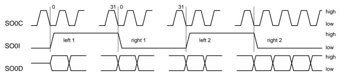
Fig. 6-2: Schematic timing of the SDO0 output interface
