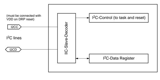
Device address: 1101010X (\$D4 (dev\_write), \$D5 dev\_read)) Slave-Subaddresses: 01101000 (\$68) subaddress write 01101001 (\$69) subaddress read 01101010 (\$6A) control
