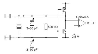
**Fig. 4–12:** Output/Input Pins 71, 72, and 74 (XTALIN, XTALOUT, AUD\_CL\_OUT)
