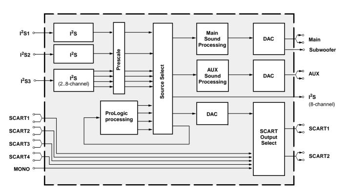
Fig. 1-1: Simplified block diagram of the DPL 4519G
