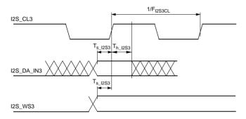
Fig. 4–22: I<sup>2</sup>S timing diagram (asynchronous interface)
