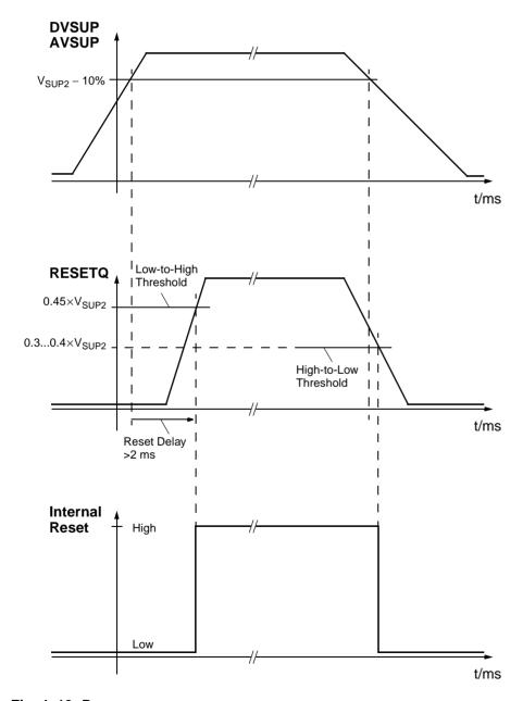
**Note:** The reset should not reach high level before the oscillator has started. This requires a reset delay of >2 ms
