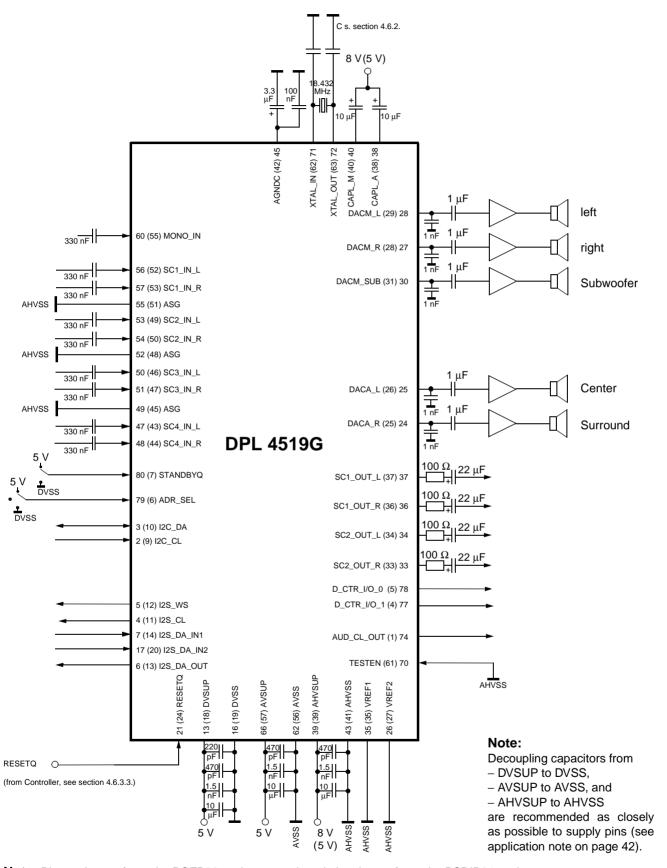
Note: Pin numbers refer to the PQFP80 package, numbers in brackets refer to the PSDIP64 package.
