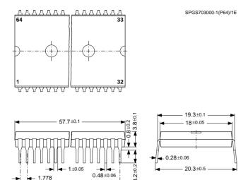
Fig. 4–3: 64-Pin Plastic Shrink Dual-Inline Package (PSDIP64) Weight approximately 9.0 g Dimensions in mm
