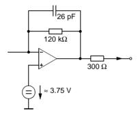
**Fig. 4–18:** Output Pins 33, 34, 36, and 37 (SC\_2\_OUT\_R/L, SC\_1\_OUT\_R/L)
