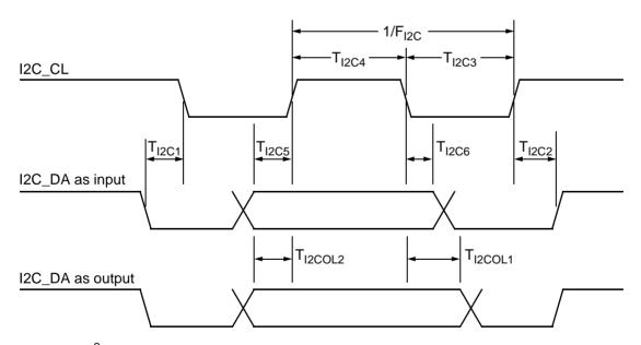
Fig. 4–20: I<sup>2</sup>C bus timing diagram
