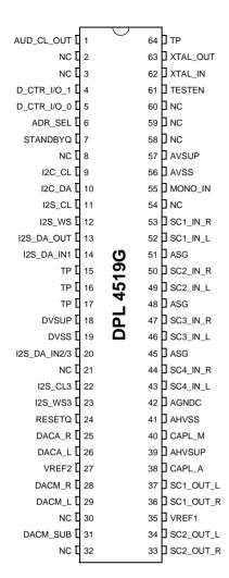
Fig. 4-6: 64-pin PSDIP package
