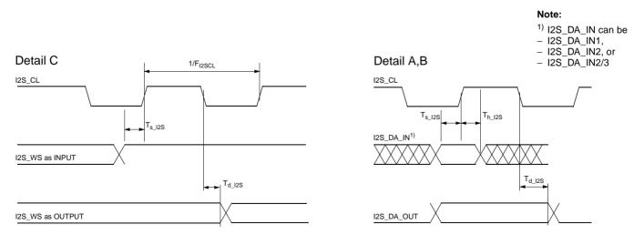
**Fig. 4–21:** I<sup>2</sup>S timing diagram (synchronous interface)
