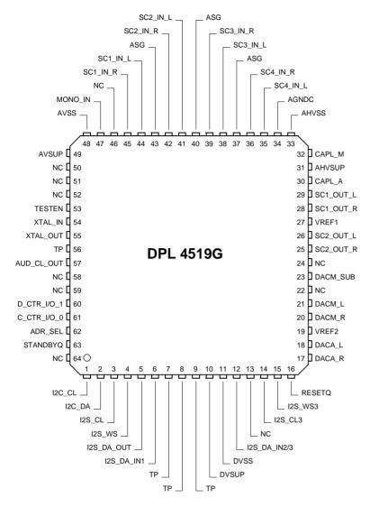
Fig. 4-5: 64-pin PLQFP package
