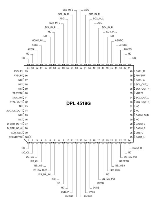
Fig. 4-4: 80-pin PQFP package
