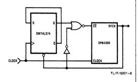
FIGURE 4b. Circuit for Extending RFCK High by 2x
