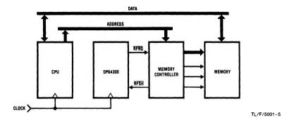
FIGURE 3a. Dynamic Memory System Using DP84300
