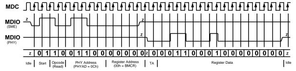
Figure 2. Typical MDC/MDIO Read Operation
