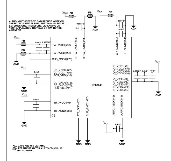
Figure 23. Power and Ground Filtering for the DP83843
