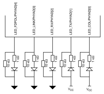
Figure 16. PHYAD Strapping and LED Loading Example
