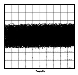
Figure 2. MLT-3 Signal Measured at All after 100 meters of CAT-5 cable
