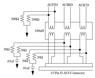
Figure 1. AUI Typical Setup
