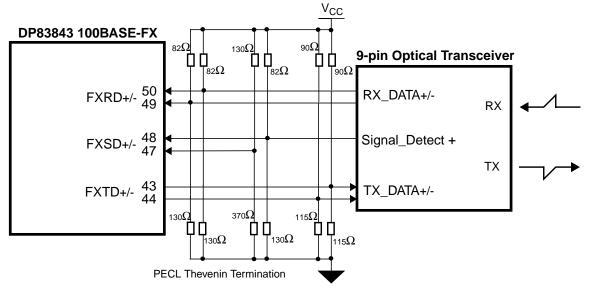
Figure 1. Typical DP83843 to Optical Transceiver Interfaces
