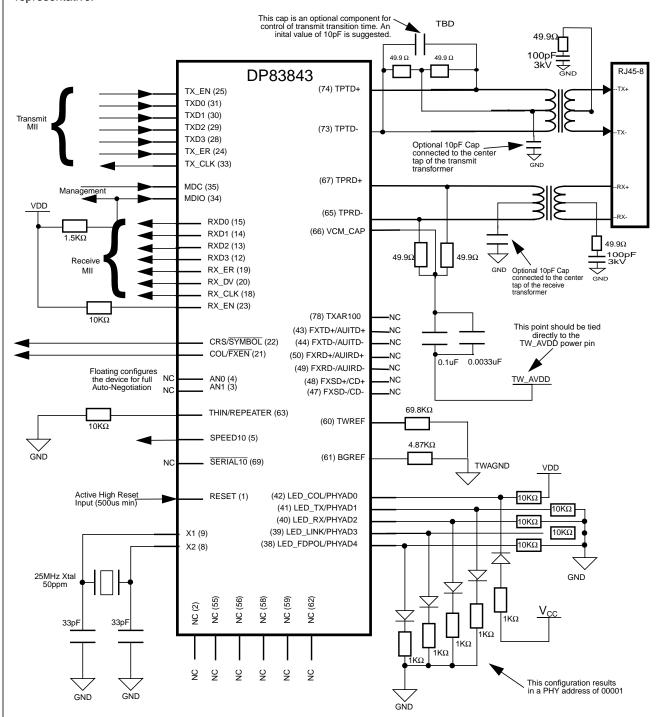
Figure 22. Typical Implementation of 10/100 Mb/s Node Application
