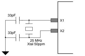
Figure 21. Xtal Reference Clock Connection Diagram
