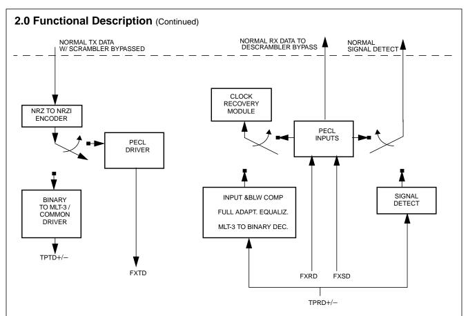
Figure 1. 100Base-FX Block Diagram
