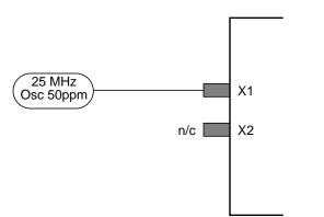
Figure 20. Oscillator Reference Clock Connection Diagram
