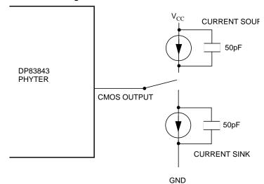
Figure 28. CMOS Output Test Load
