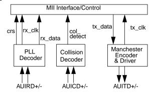
Figure 1. AUI Block Diagram
