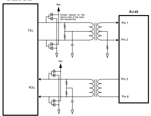
Figure 25. Typical DP83843 Network Interface with additional ESD protection
