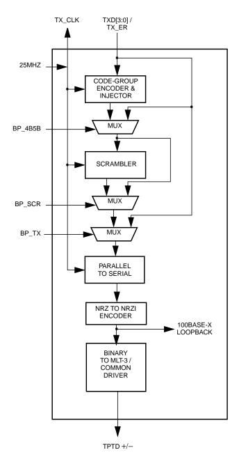
Figure 1. 100BASE-TX Transmit Block Diagram
