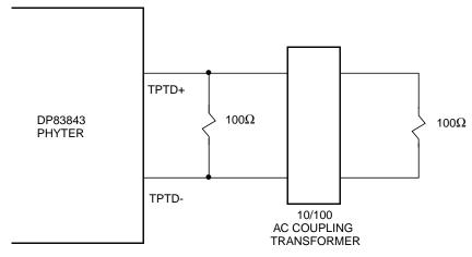
Figure 29. 10/100 Twisted Pair Load (zero meters)
