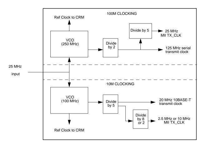
Figure 17. Clock Generation Module BLOCK DIAGRAM
