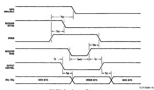
FIGURE 8. Error Sequence Timing
