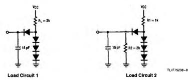
FIGURE 6. Test Load Circuits
