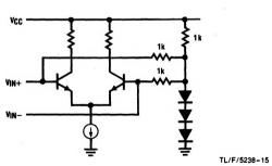
FIGURE 13. Equivalent Circuit for DP8341/NS32441 Input Amplifier
