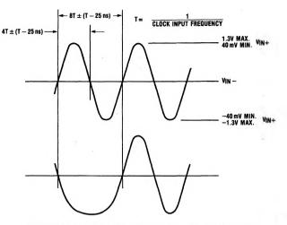
FIGURE 10. Data Waveform Constraints: Amplifier Inputs
