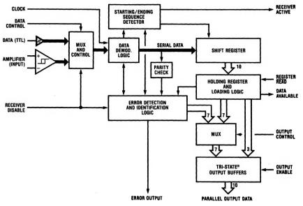
FIGURE 2. DP8341/NS32441 Serial Bi-Phase Receiver/Decoder Block Diagram
