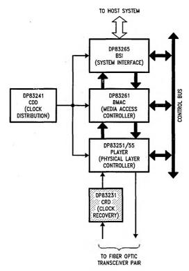
FIGURE 1-1. FDDI Chip Set Block Diagram
