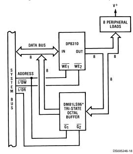
\*High Level Input Voltage must not Exceed V<sub>CC</sub> of the DM81LS96
