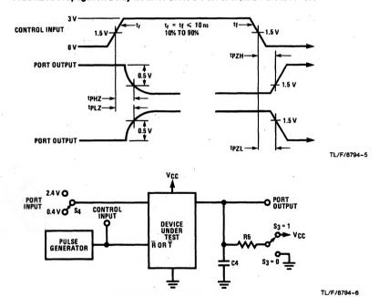
Note: C4 includes test fixture capacitance. Port input is in a fixed logical condition. See AC Table.
