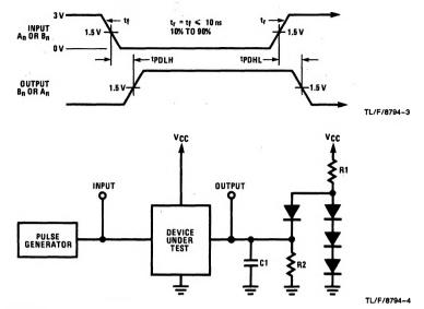
Note: C1 includes test fixture capacitance.
