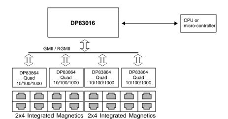
Targeted at desktop/workgroup LAN connectivity, the DP83016 offers new levels of integration and performance for Gigabit Ethernet switch applications.
