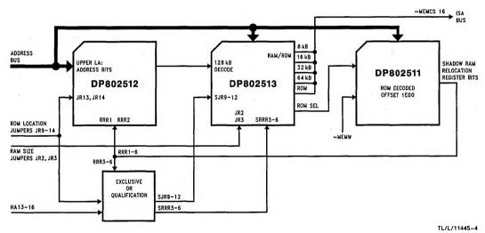
FIGURE 2. MEMCS\_Logic
