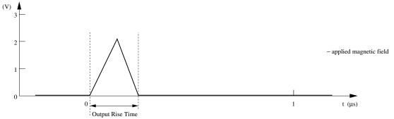
$V_{CC}$  = 3.0 V, Pull-Up-R. = 56  $\mathrm{k}\Omega$
