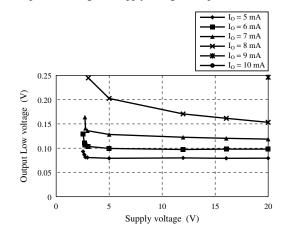
Output low voltage — Supply voltage (Temp. =  $25^{\circ}$ C)
