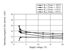
Operating magnetic flux density — Supply voltage
