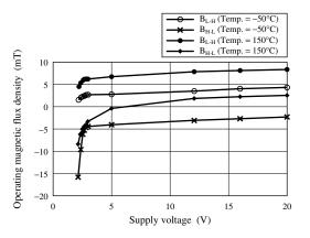
Operating magnetic flux density — Supply voltage
