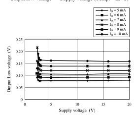
Output low voltage — Supply voltage (Temp. = 150°C)
