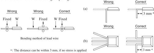
\*: The distance can be within 3 mm, if no stress is applied to the resin mold by tightly fixing the lead wires with a metallic mold or the like.
