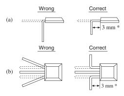
Bending position of lead wire
