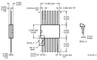
14-Lead Ceramic Flat Package (W) Order Number 5473FMQB or DM5473W Package Number W14B
