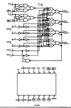
outputs is actually (Complement A  $\oplus$  Data A). That this is the case may be verified by examining the logic diagram.
