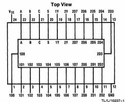
Order Number DM54LS451AJ, DM74LS451AJ, DM74LS451AN or DM74LS451AV See NS Package Number J24F, N24C or V28A
