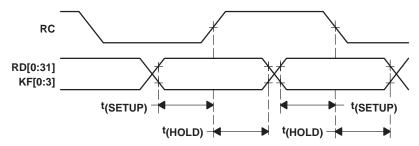
Figure 8. Receive Interface Timing
