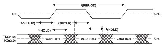
Figure 14. XGMII Transmit Timing Diagram
