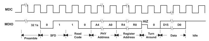
Figure 10. Management Interface Read Timing
