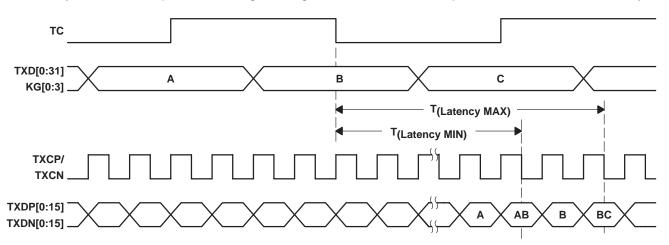
Figure 6. Transmitter Latency
