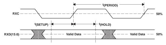
Figure 13. XSBI Receive Timing Diagram
