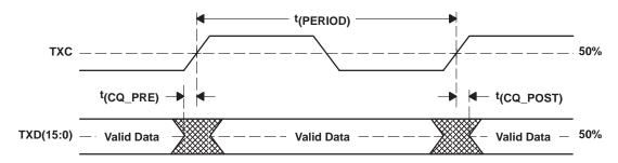
Figure 12. XSBI Transmit Timing Diagram
