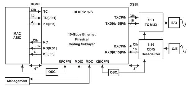
Figure 1. 10-Gbps Ethernet Short-PCB-Distance Implementation
