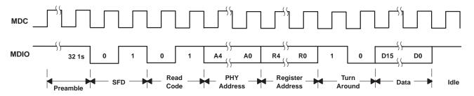
Figure 11. Management Interface Write Timing
