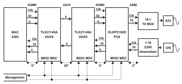
Figure 2. 10-Gbps Ethernet Long-PCB-Distance Implementation
