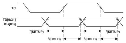
Figure 4. XGMII Transmit Timing
