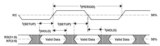
Figure 15. XGMII Receive Timing Diagram
