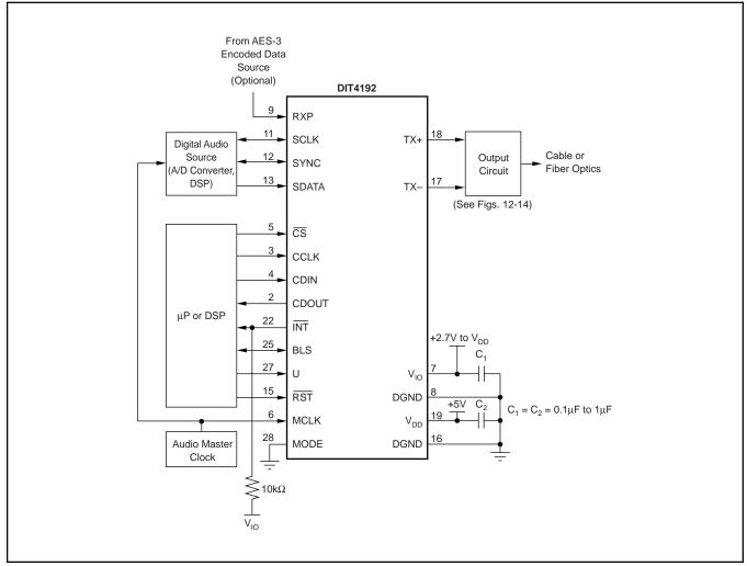
FIGURE 10. Typical Circuit Configuration, Software Mode.
