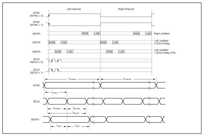
FIGURE 4. Audio Data Formats and Timing.
