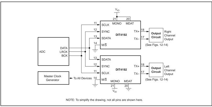
FIGURE 15. Hardware Mode Example for Dual-Channel Transmitter Operation.
