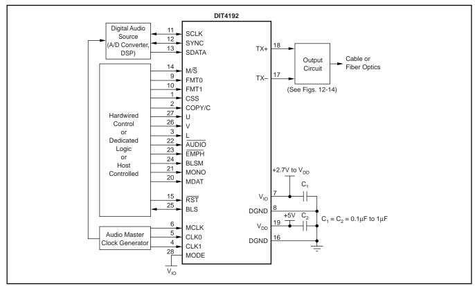
FIGURE 11. Typical Circuit Configuration, Hardware Mode.
