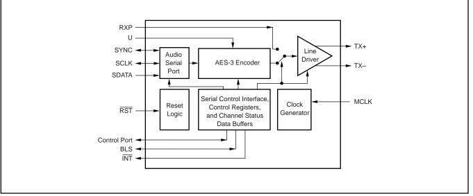
FIGURE 1. Software Mode Block Diagram.
