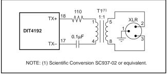
FIGURE 12. Recommended Transmitter Output Circuit for Balanced,  $110\Omega$  Twisted-Pair Transmission.
