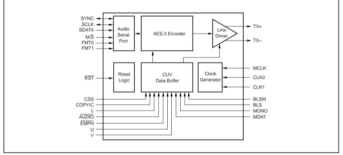
FIGURE 2. Hardware Mode Block Diagram.
