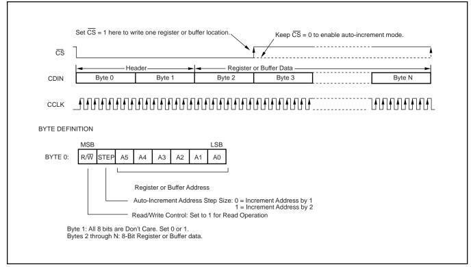
FIGURE 6. Write Operation Format.
