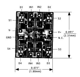
TRANSISTOR COUNT: 126 SUBSTRATE CONNECTED TO V+
