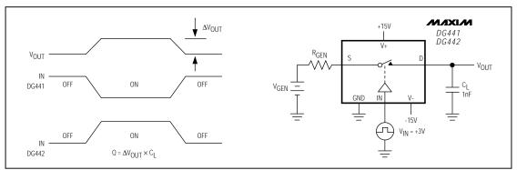
Figure 3. Charge Injection
