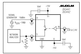
Figure 4. Off-Isolation Rejection Ratio
