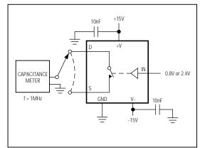
Figure 6. Source/Drain-On/-Off Capacitance
