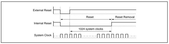
FIGURE 3. External Forces Reset Timing.
