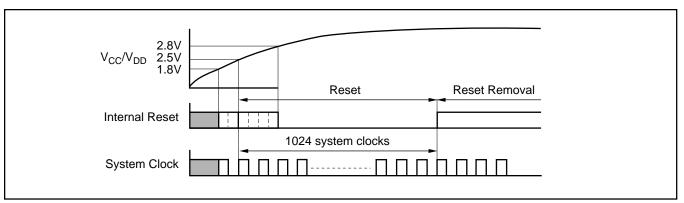
FIGURE 2. Internal Power-On Reset Timing.
