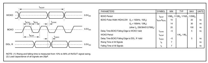
FIGURE 7. Audio Data Output Timing.
