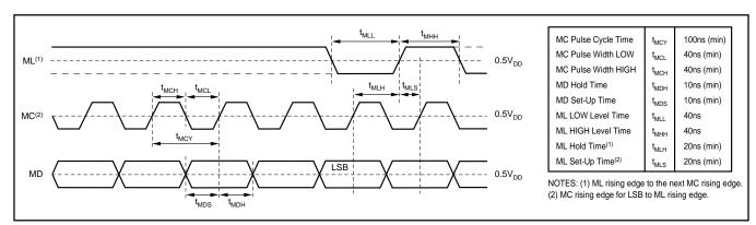
FIGURE 10. Software Interface Timing Requirements.
