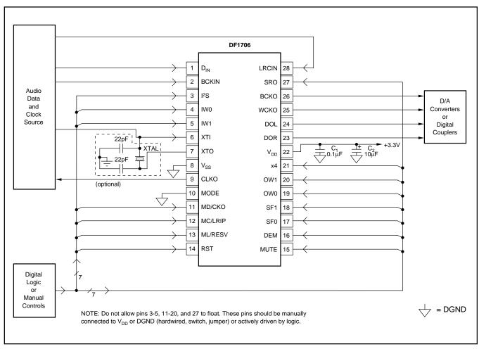
FIGURE 12. Basic Circuit Connections, Hardware Control.
