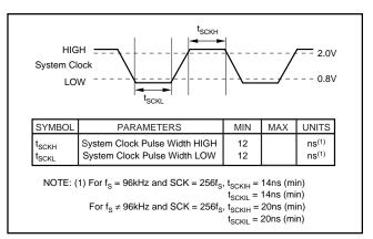
FIGURE 1. System Clock Timing.
