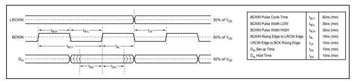
FIGURE 5. Audio Input Interface Timing.
