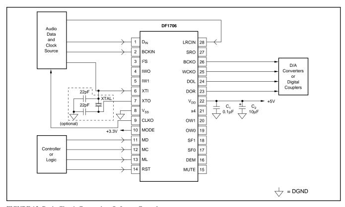
FIGURE 13. Basic Circuit Connection, Software Control.
