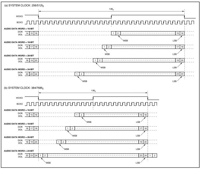
FIGURE 6. Audio Output Data Format.
