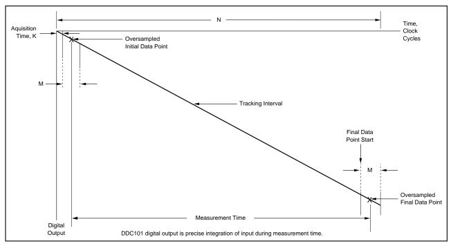
FIGURE 11. Equivalent Integrator Output for Single Integration.
