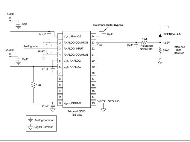
FIGURE 24. Example of Basic DDC101 Circuit Connections.
