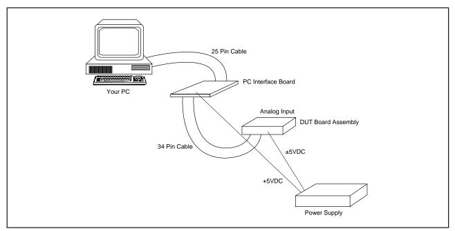
FIGURE 29. DEM-DDC101P-C Evaluation Fixture Connection Diagram.
