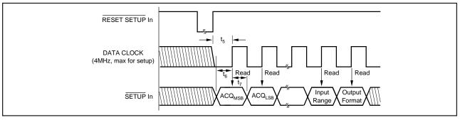
FIGURE 5. Input/Output Timing Diagram—SETUP Timing Diagram.
