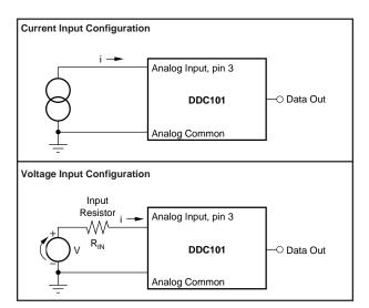
FIGURE 9b. DDC101 Input Configurations.
