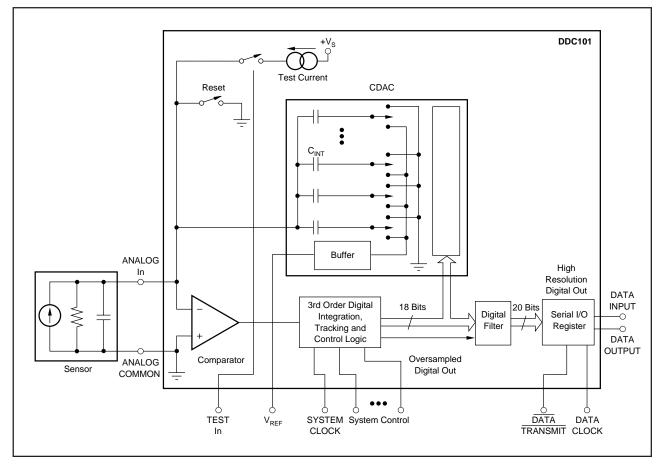
FIGURE 3. DDC101 Detailed Circuit Diagram.
