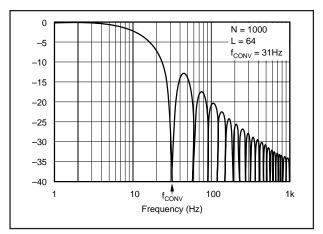
FIGURE 18. A Multiple Integration Frequency Response Example.
