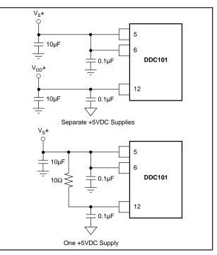
FIGURE 23. Positive Supply Connection Options.
