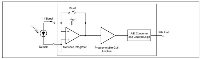
FIGURE 1. Simplified Equivalent Circuit of DDC101 to Illustrate Function.
