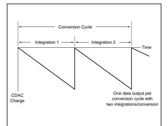
FIGURE 15. Conversion Cycle with Two Integrations.
