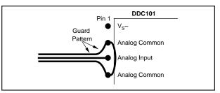
FIGURE 22. PC Board Layout Showing "Guard" Traces Surrounding Analog Input Pin and Traces.
