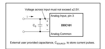
FIGURE 9a. Current Pulse Input Capture.
