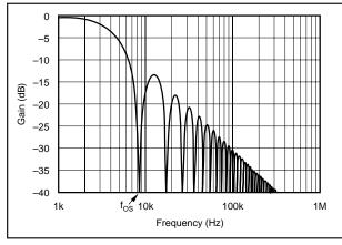
FIGURE 17. Oversampling Frequency Response for M = 256( $f_{CLK} = 2MHz$ ).
