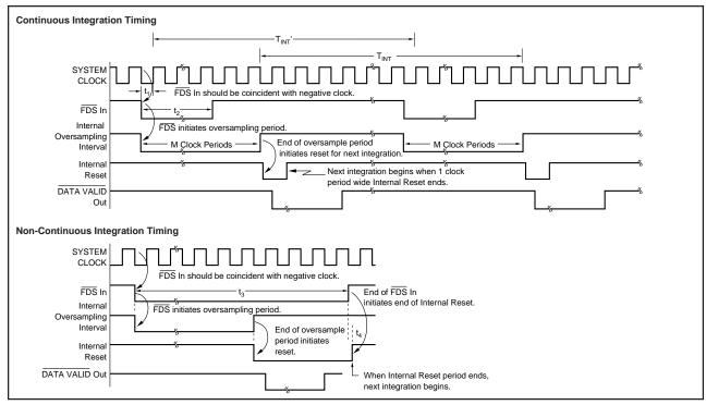
FIGURE 4. Conversion Timing Diagrams.
