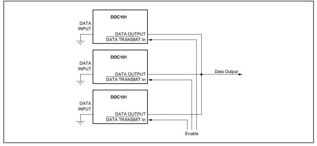
FIGURE 27. DDC101 Parallel Operation.
