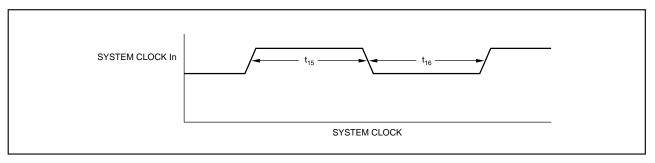
FIGURE 8. System Clock Timing.
