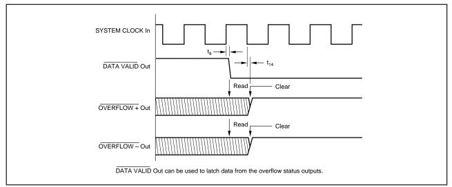
FIGURE 7. OVERFLOW Out Monitoring Timing Diagram.
