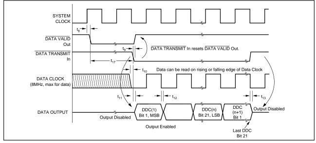
FIGURE 6. DATA TRANSMIT Timing Diagram.
