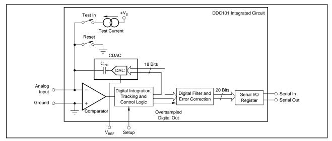
FIGURE 2. DDC101 Block Diagram.
