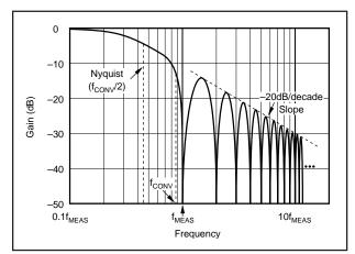
FIGURE 16. Basic Integration Frequency Response.
