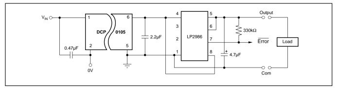
FIGURE 10. Post Regulation of DCP010505P.
