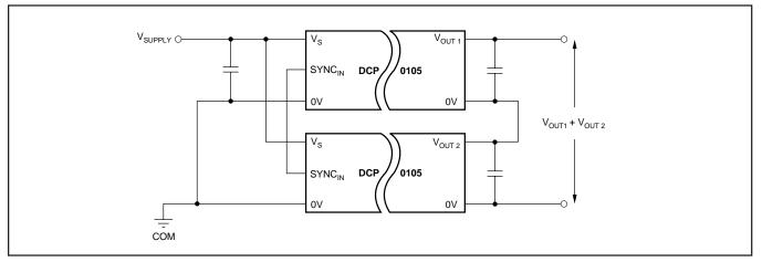
FIGURE 4. Connecting the DCP0105 in Series.
