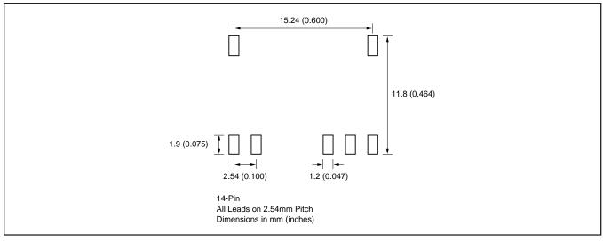
FIGURE 11. PCB Pad Size and Placement for "U" Package.
