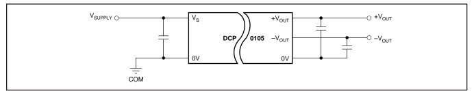
FIGURE 5. Connecting Dual Outputs in Series.
