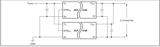
FIGURE 6. Connecting Multiple DCP0105s in Parallel.
