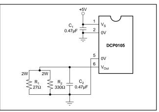
FIGURE 2. DCP010505 Fully Loaded.
