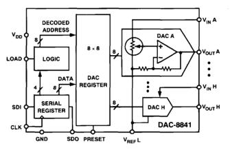
The DAC-8841 consumes only 95 mW from a +5 V power supply. For dual polarity applications see the DAC-8840 which provides full 4-quadrant-multiplying  $\pm 3$  V signal capability while operating from  $\pm 5$  V power supplies.
