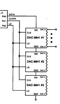
Figure 21. Three-Wire Interface
