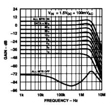
Figure 22. Gain ( $V_{OUT}/V_{IN}$ ) and Feedthrough vs. Frequency
