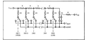
FIGURE 2: N-Channel Current Steering Switch
