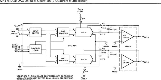
FIGURE 4: Dual DAC Unipolar Operation (2-Quadrant Multiplication)
