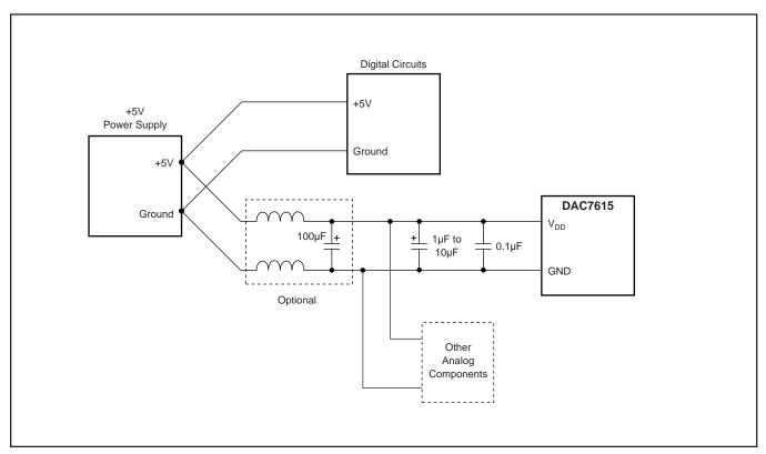
FIGURE 4. Suggested Power and Ground Connections for a DAC7615 Sharing a +5V Supply with a Digital System.
