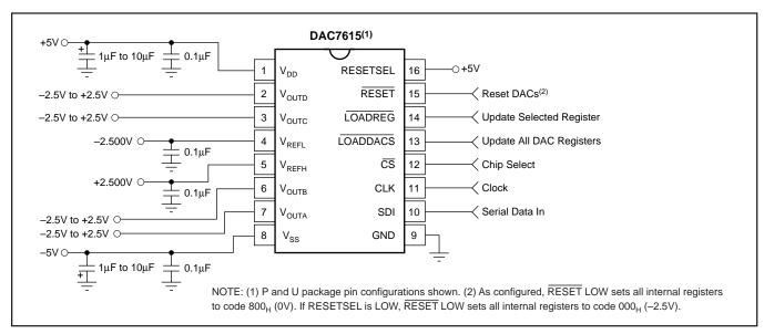
FIGURE 2. Basic Dual-Supply Operation of the DAC7615.
