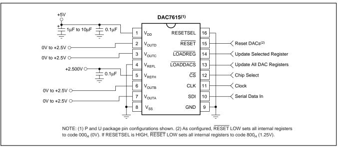
FIGURE 1. Basic Single-Supply Operation of the DAC7615.
