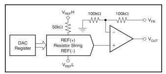
Figure 26. Typical DAC Architecture
