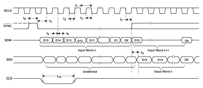
Figure 1. Serial Write Operation Timing Diagram
