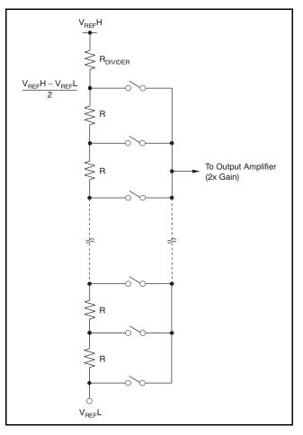
Figure 27. Typical Resistor String
