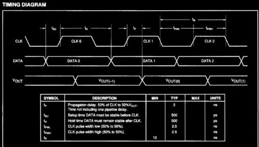
NOTE: Timing is specified in the mode with the LATCH mode floating.
