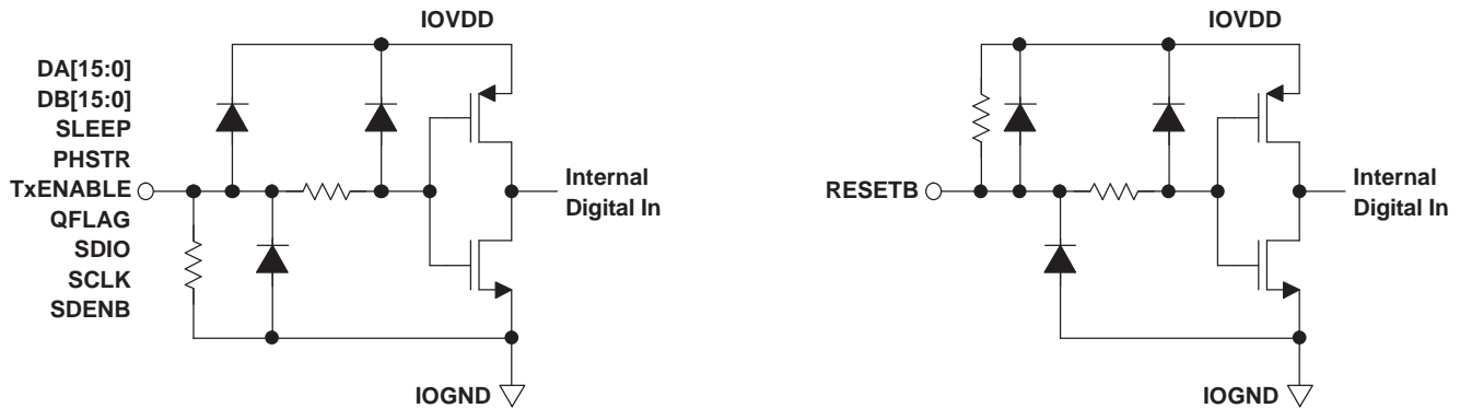
Figure 61. CMOS/TTL Digital Equivalent Input
