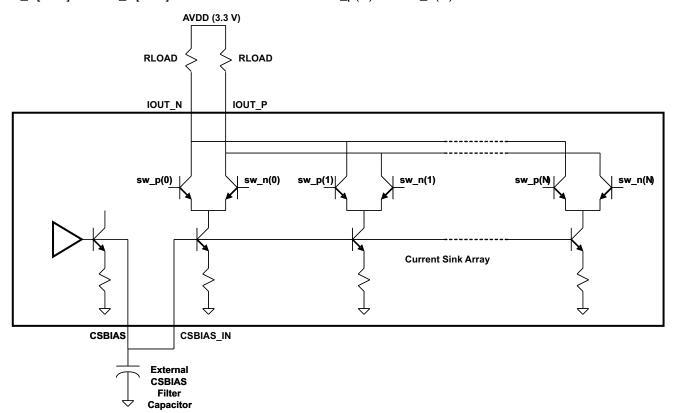
Figure 25. Current Sink Array
