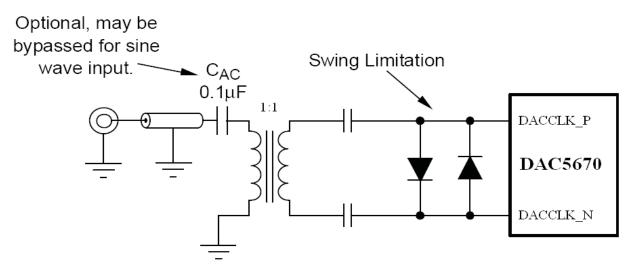
Figure 19. Driving the DAC5670 with a Single-Ended Clock Source Using a Transformer
