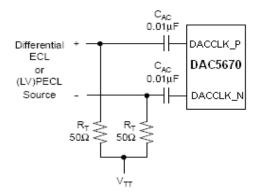
Figure 21. Driving the DAC5670 with a Differential ECL/PECL Clock Source
