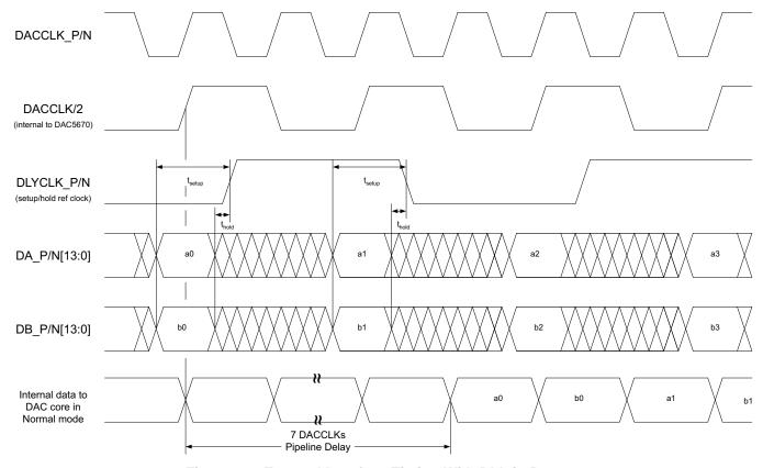
Figure 17. External Interface Timing With DLL in Restart
