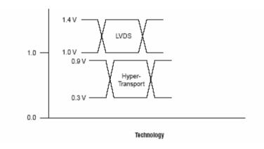
Figure 11. Digital Input Voltage Options
