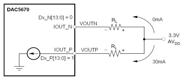
Figure 23. Relationship between D[13:0], IOUT N and IOUT P
