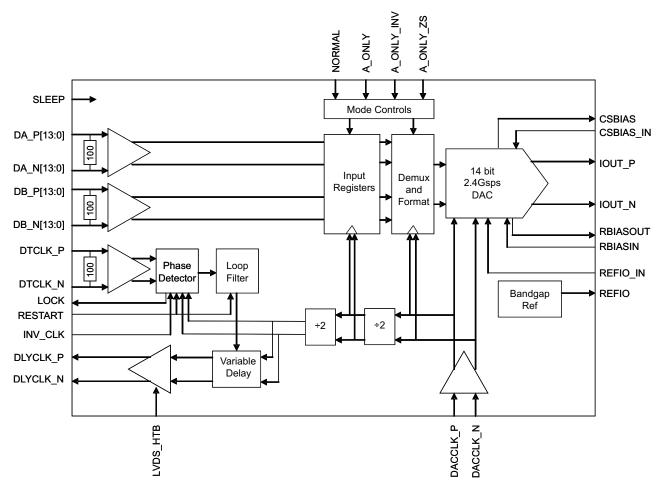
Figure 1. Functional Block Diagram DAC5670
