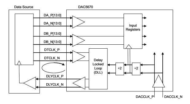
Figure 14. DLL Input Loop Simplified Block Diagram
