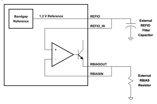
Figure 24. Reference Circuit
