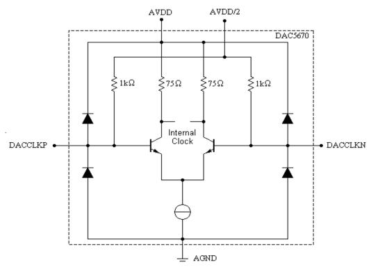
Figure 18. Clock Equivalent Input
