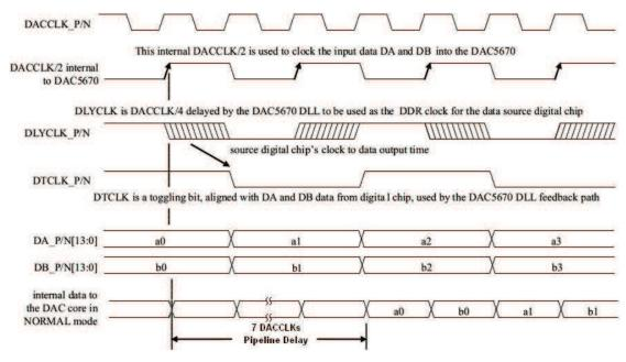
Figure 16. DLL Input Loop Functional Timing
