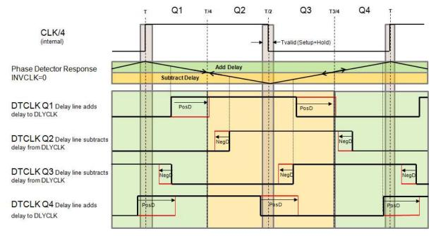
Figure 15. DLL Phase Detector Behavior
