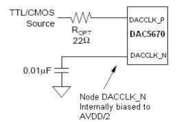
Figure 22. Driving the DAC5670 with a Single-Ended TTL/CMOS Clock Source
