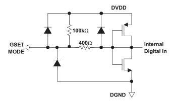
Figure 16. CMOS/TTL Digital Equivalent Input With Internal Pullup Resistor
