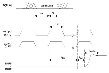
Figure 17. Dual Bus Mode Operation
