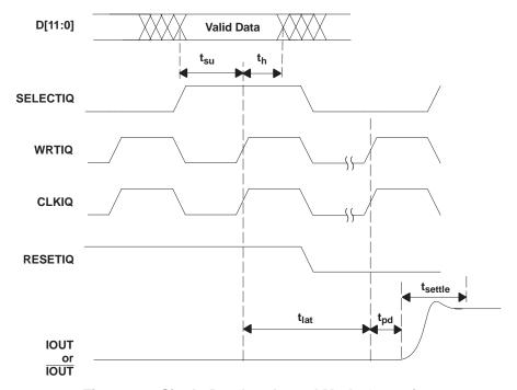
Figure 18. Single-Bus Interleaved Mode Operation
