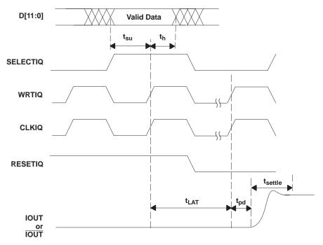
Figure 19. Single-Bus Interleaved-Mode Operation
