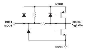
Figure 15. CMOS/TTL Digital Equivalent Input With Internal Pullup Resistor
