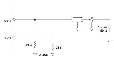
Figure 21. Driving a Doubly-Terminated 50- $\Omega$  Cable Using a Single-Ended Output
