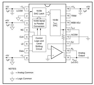
FIGURE 2. Connection Diagram.
