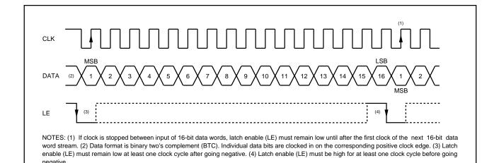
FIGURE 4. Input Timing Diagram.
