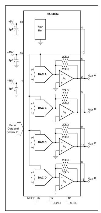
FIGURE 5. Analog Connections for 0 to –10V DAC Output.
