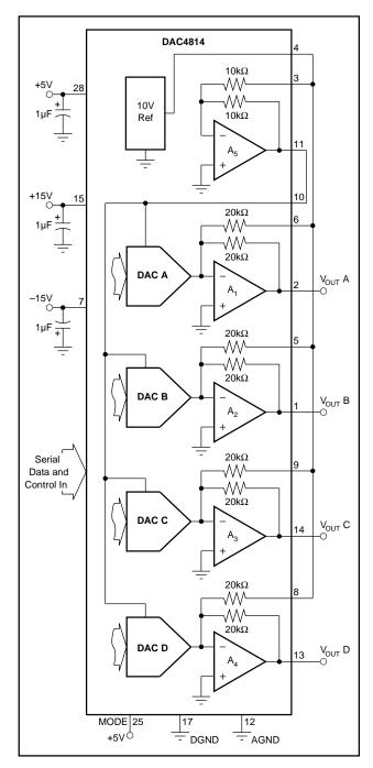
FIGURE 3. Analog Connections for ±10V DAC Output.
