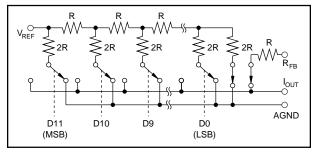
FIGURE 1. Simplified Circuit Diagram of DAC Cell.
