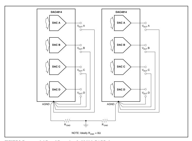
FIGURE 2. Recommended Ground Connections for Multiple DAC Packages.
