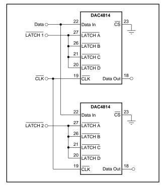
FIGURE 7. Parallel Bus Connection for Multiple DAC Packages.
