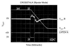
NOTE: Crosstalk is dominated by digital crosstalk/feedthrough of the  $\overline{\text{LATCH}}$  signal.
