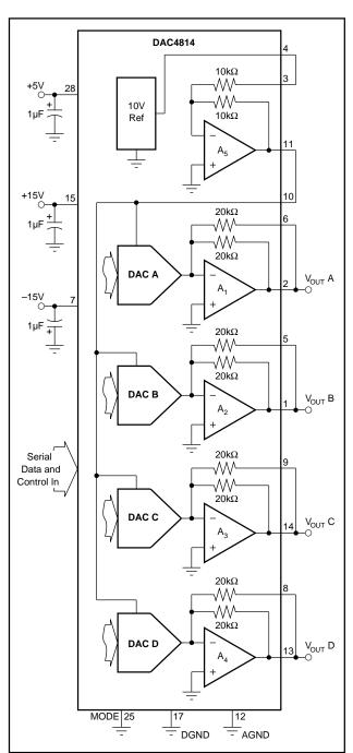
FIGURE 4. Analog Connections for 0 to +10V DAC Output.
