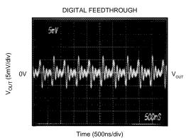
DAC output noise due to activity on digital inputs with latch disabled.
