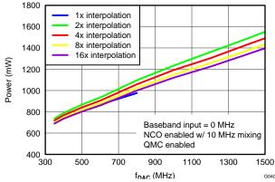
Figure 40. Power vs f<sub>DAC</sub> Over Interpolation
