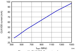
Figure 46. CLKVDD Current vs f<sub>DAC</sub>
