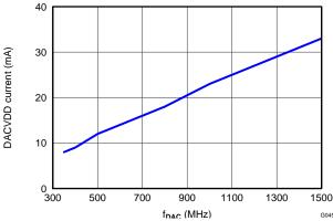
Figure 45. DACVDD Current vs f<sub>DAC</sub> Over Interpolation
