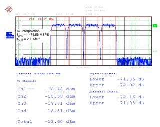
Figure 34. Four-Carrier WCDMA Test Mode1
