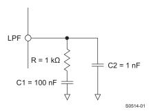
Figure 57. Recommended External Loop Filter
