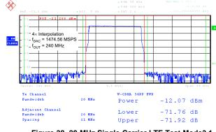
Figure 38. 20-MHz Single-Carrier LTE Test Mode3.1
