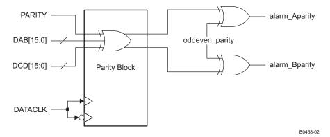
Figure 79. DAC34SH84 32-Bit Parity Check
