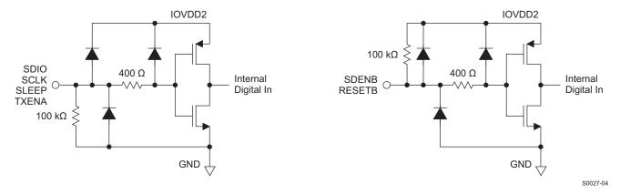
Figure 85. CMOS Digital Equivalent Input
