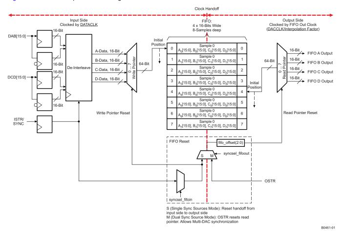
Figure 52. DAC34SH84 FIFO Block Diagram
