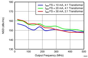
Figure 25. NSD vs Output Frequency Over  $I_{OUT}FS$
