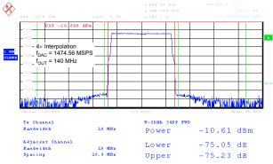
Figure 35. 10-MHz Single-Carrier LTE Test Mode3.1
