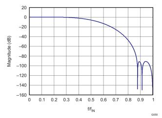
Figure 64. Magnitude Spectrum for FIR2
