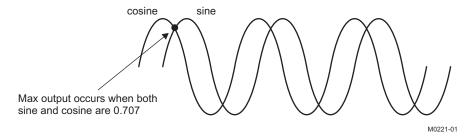
Figure 74. Maximum Output of the Complex Signal Multiplier
