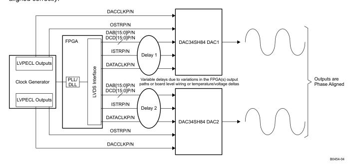
Figure 58. Synchronization System in Dual Sync Sources Mode With PLL Bypassed
