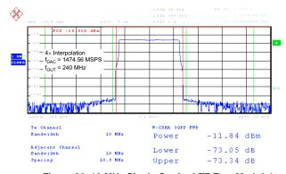
Figure 36. 10-MHz Single-Carrier LTE Test Mode3.1
