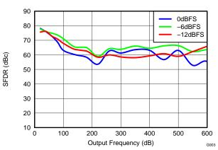
Figure 3. SFDR vs Output Frequency Over Input Scale
