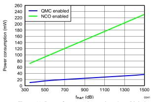
Figure 41. Power Consumption vs f<sub>DAC</sub> Over Digital Processing Functions
