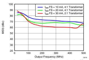
Figure 18. IMD3 vs Output Frequency Over I<sub>OUT</sub>FS
