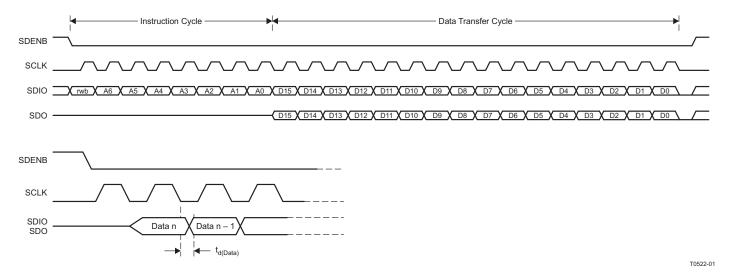
Figure 50. Serial-Interface Read Timing Diagram
