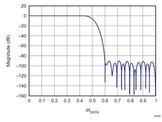
Figure 66. 2x Interpolation Composite Response
