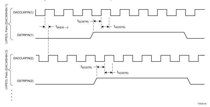
Figure 59. Timing Diagram for LVPECL Synchronization Signals
