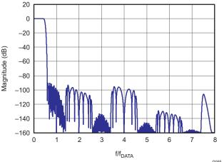
Figure 68. 8x Interpolation Composite Response
