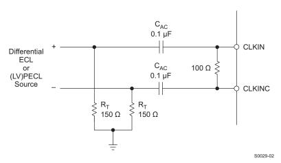
Figure 82. Preferred Clock Input Configuration With a Differential ECL or PECL Clock Source
