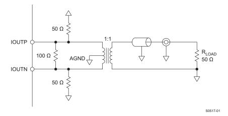
Figure 86. Driving a Doubly Terminated 50 Ω Cable Using a 1:1 Impedance Ratio Transformer
