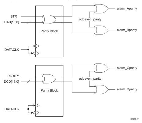
Figure 80. DAC34SH84 Dual 16-Bit Parity Check
