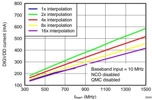
Figure 43. DIGVDD Current vs f<sub>DAC</sub> Over Interpolation
