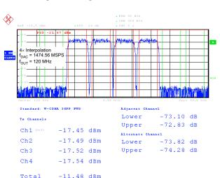
Figure 33. Four-Carrier WCDMA Test Mode1
