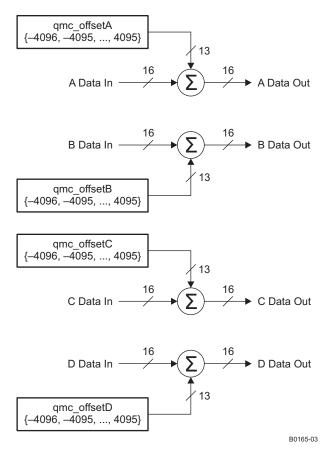
Figure 76. Digital Offset Block Diagram
