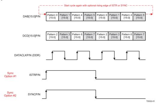
Figure 77. I/O Pattern Checker Data Transmission Format
