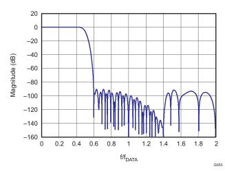
Figure 67. 4x Interpolation Composite Response
