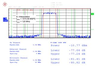
Figure 30. Single-Carrier WCDMA Test Mode1
