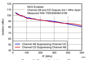
Figure 48. Channel Isolation vs IF
