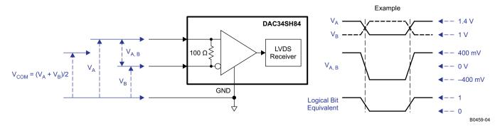
Figure 84. LVDS Data Input Levels
