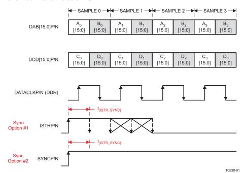
Figure 51. Data Transmission Format
