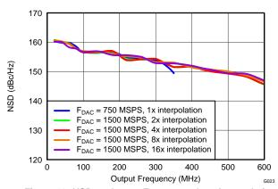
Figure 23. NSD vs Output Frequency Over Interpolation
