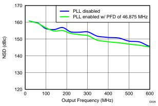
Figure 26. NSD vs Output Frequency Over Clocking Options
