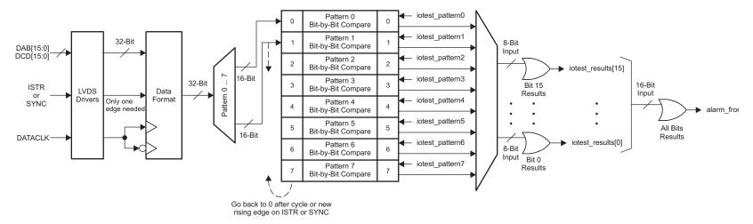
Figure 78. DAC34SH84 Pattern Check Block Diagram
