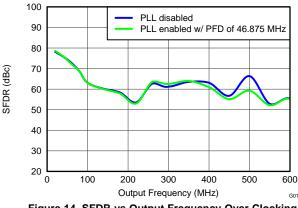
Figure 14. SFDR vs Output Frequency Over Clocking Options
