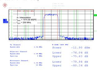
Figure 31. Single-Carrier WCDMA Test Mode1
