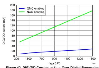
Figure 42. DIGVDD Current vs f<sub>DAC</sub> Over Digital Processing Functions
