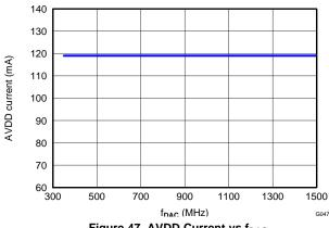
Figure 47. AVDD Current vs f<sub>DAC</sub>
