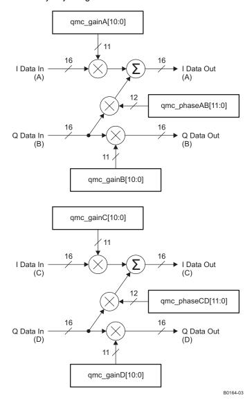
Figure 75. QMC Block Diagram
