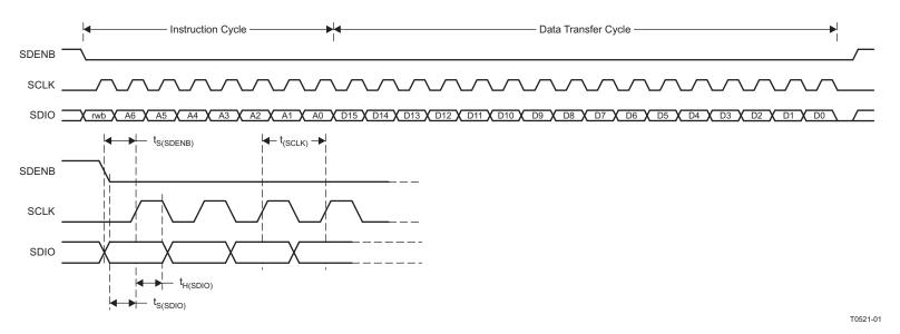
Figure 49. Serial-Interface Write Timing Diagram
