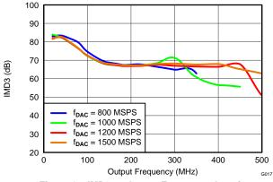
Figure 17. IMD3 vs Output Frequency Over f<sub>DAC</sub>
