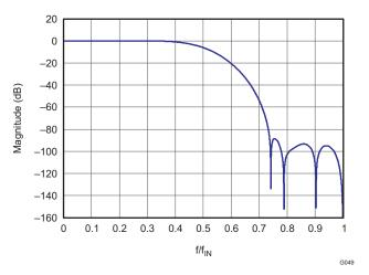
Figure 63. Magnitude Spectrum for FIR1
