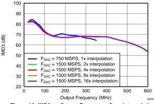
Figure 16. IMD3 vs Output Frequency Over Interpolation
