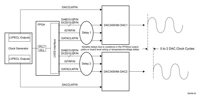
Figure 61. Multi-Device Operation in Single Sync Source Mode
