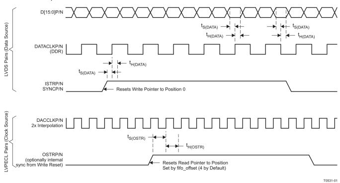
Figure 53. FIFO Write and Read Descriptions
