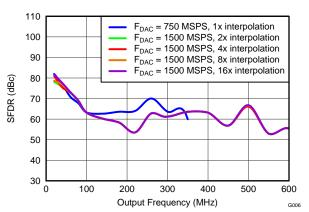
Figure 6. SFDR vs Output Frequency Over Interpolation
