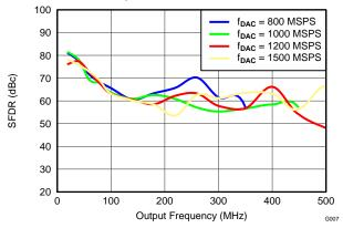
Figure 7. SFDR vs Output Frequency Over fDAC
