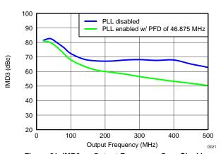
Figure 21. IMD3 vs Output Frequency Over Clocking Options
