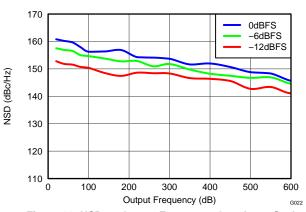
Figure 22. NSD vs Output Frequency Over Input Scale
