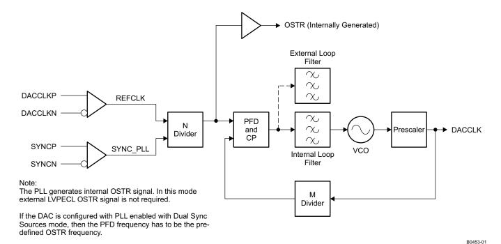
Figure 55. PLL Block Diagram
