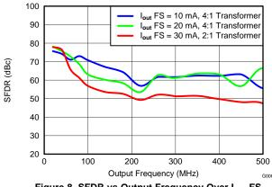
Figure 8. SFDR vs Output Frequency Over I<sub>OUT</sub>FS
