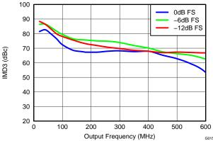
Figure 15. IMD3 vs Output Frequency Over Input Scale
