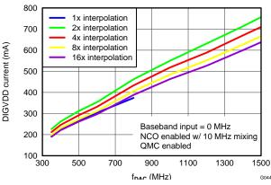
Figure 44. DIGVDD Current vs f<sub>DAC</sub> Over Interpolation
