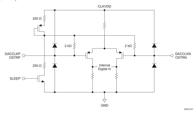
Figure 81. DACCLKP/N and OSTRP/N Equivalent Input Circuit
