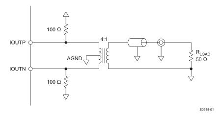
Figure 87. Driving a Doubly Terminated 50  $\Omega$  Cable Using a 4:1 Impedance Ratio Transformer
