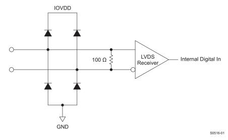
Figure 83. DAB[15:0]P/N, DCD[15:0]P/N, DATACLKP/N, ISTRP/N, SYNCP/N and PARITYP/N LVDS Input Configuration
