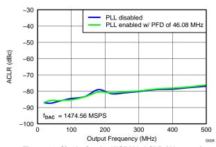
Figure 28. Single-Carrier WCDMA ACLR (Alternate) vs Output Frequency Over Clocking Options
