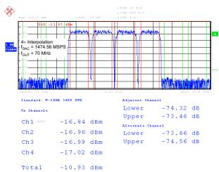
Figure 32. Four-Carrier WCDMA Test Mode1
