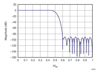
Figure 62. Magnitude Spectrum for FIR0
