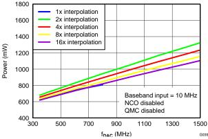
Figure 39. Power vs f<sub>DAC</sub> Over Interpolation
