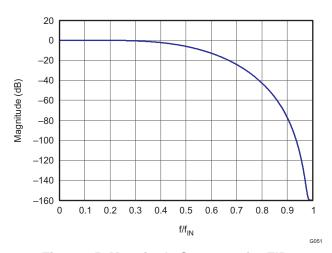
Figure 65. Magnitude Spectrum for FIR3
